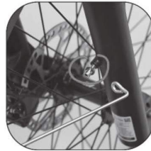
Installing the fenders on the shocks (Shocks come with screws and spacers)
