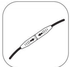
Look closely and you can see the arrows in the joint, arrow to arrow connection
