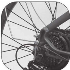
Rear fenders mounted underneath (It's the same on the other side.)
